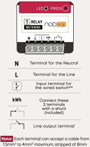
\*\*Wired switch optional (see the installation diagrams section on the next page)
